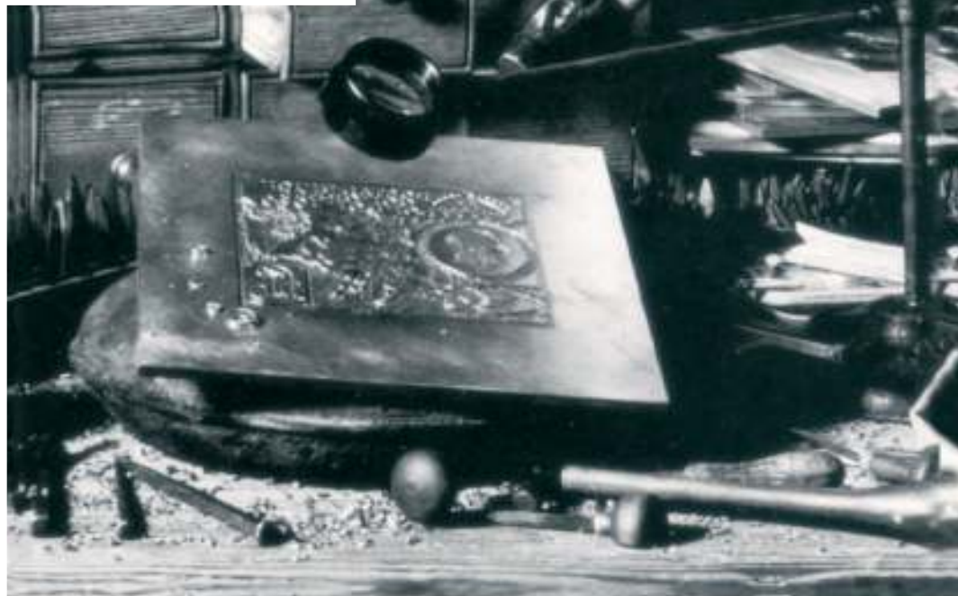
Enlarged illustration to show the fine detailing which can only be achieved by traditional craftsmanship. The serrated edges are a full 2.2 mm thick.
